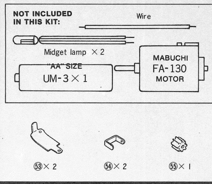
Due to the *optional* motorization capabilities designed into this kit, you will find certain parts and assembly steps included within this kit — and instruction sheet — that apply directly to mounting a motor and batteries (not included), on-off switch and wiring.
