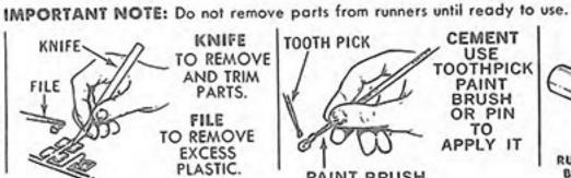
KNIFE TO REMOVE AND TRIM PARTS. TO REMOVE EXCESS
